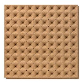
**MOUNTING CONDITIONS** Undertone modified coating, cork and the base area average drilling of 4.96%, installed on structure in metallic profiles, creating an air box with a thickness of about 70mm partially filled with mineral wool with thickness nominal of 40mm.
