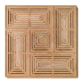
**MOUNTING CONDITIONS** Buzzer coating, cork-based with ribs / grooves, installed on structure in metal profiles, creating an air box with a thickness of about 70mmpartially filled with mineral wool with nominal thickness of 40mm.
